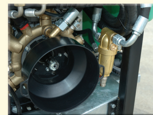
Filtro in mandata in ottone Brass delivery filter
